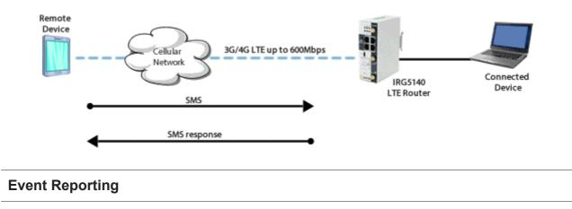
The IRG5140 Router can be configured to generate reports, or initiate actions, based on specified events. These events can be generated internally, or externally by devices attached to the IRG5140 digital inputs or alarm relay.
